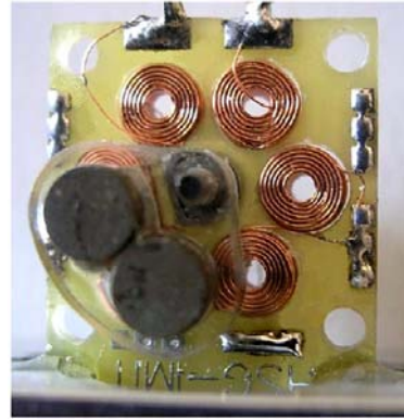
Fig. 10. Generator converts vibration to rotation.
